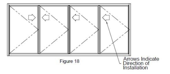
The mullion center lines must be laid out before the first window can be installed. Take into account the 3/16" shim at the extreme jambs and the leg engagement at the vertical mullion. The vertical mullion is designed to be set flush with the interior side of the storefront frame. This is necessary to position the vent glass in the same plane as the storefront glass.
